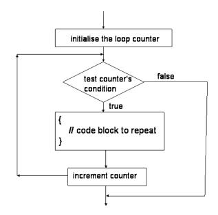
Figure 2.5 Counter-controlled repetition of a block of code
