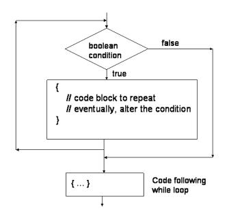
Figure 2.6 The logic of a while loop
