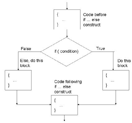
Figure 2.1 The logic of the if ... else construct
