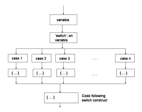
Figure 2.3 The logic of the switch ... case construct
