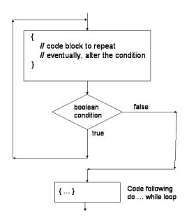
Figure 2.7 The logic of a do ... while loop
